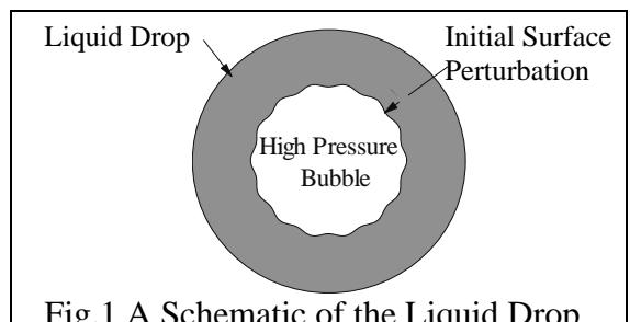
Fig.1 A Schematic of the Liquid Drop
