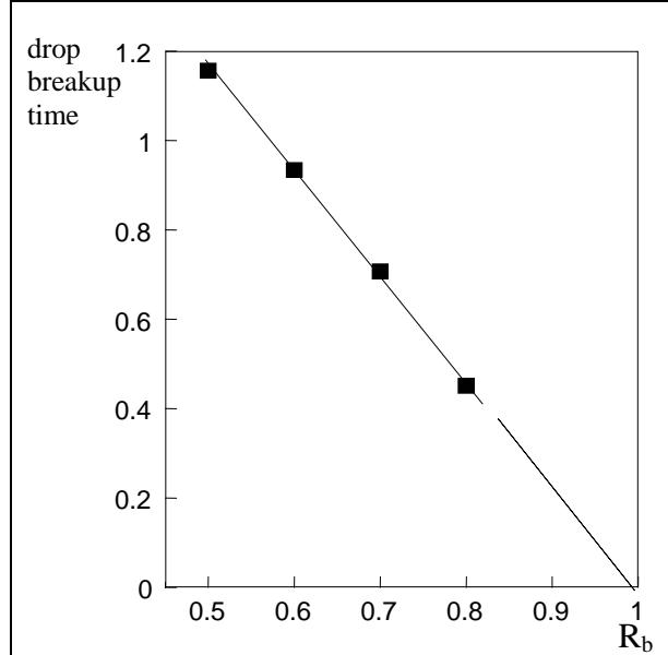
Fig. 7 Drop breakup time as a function of initial bubble radius
