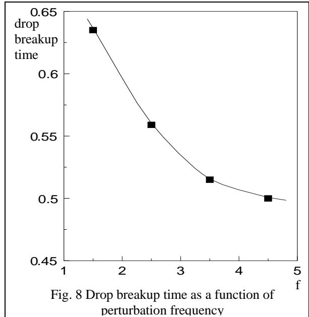
Fig. 8 Drop breakup time as a function of perturbation frequency
