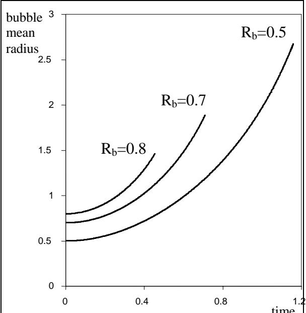
Fig. 6 Bubble growth rate at different initial bubble radii
