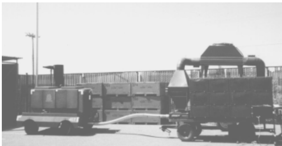
Figure 11: NO x filter cart for diesel exhaust capture
